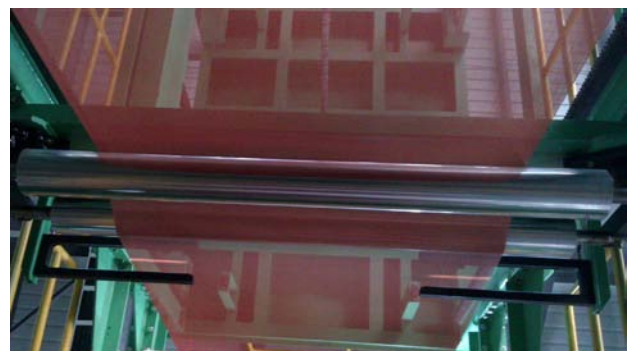
Photoelectric Center Sensors DCP-450 are used with a End Pivot Guide
